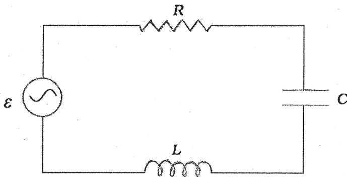
Figure shows a ideal series LCR circuit connected to a.c. mains of voltage  $\epsilon$ ,
