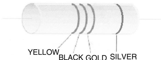
What is the value of the resistor ? What is its tolerance ? Why are carbon resistors preferred in most electronic circuits ?
